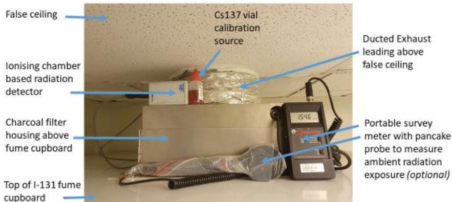
Radiation detector being tested with sealed Cs137 vial source during annual check
